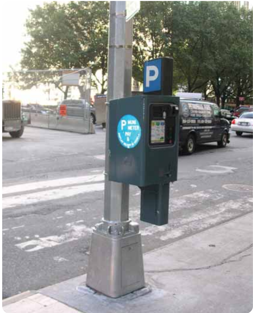
The NYC Bureau of Parking developed a way to attach P and D machines to the light standards. This leads to much less street furniture and a dramatically improved streetscape. The unit is powered through the lighting system.
