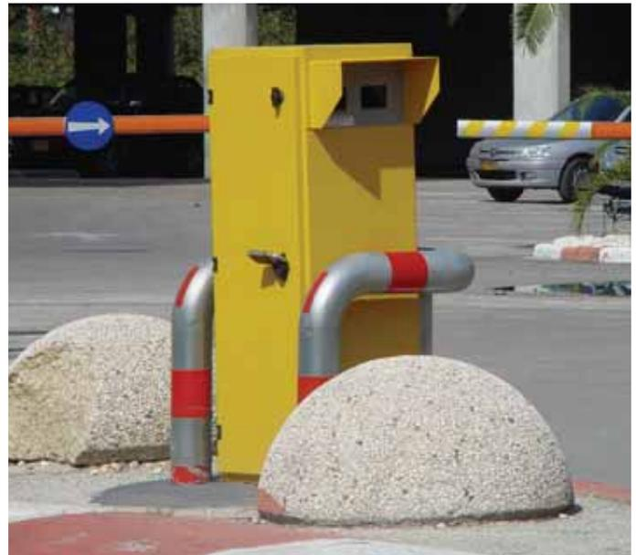
Automatic License Plate Recognition systems are intended to eliminate losses caused by parking “cheaters”.
