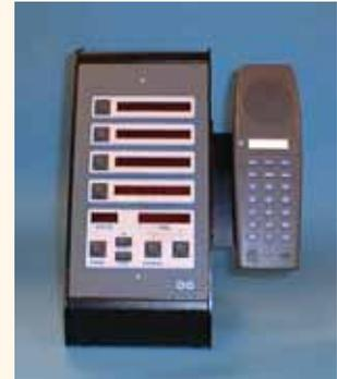
The incoming calls will display in a 12 character Alphanumeric message on the Digital Annunciator Display module. There are 9 levels of assignable priority for each and every call to ensure that the highest risk calls will be displayed at the top of the display.
